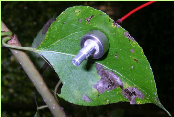
Fig. 4: ZIM-magnet probe for leaf-potential measurement (turgor) at poplar
