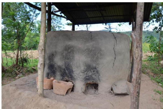
Figure 7: The kiln in which the clay liners are burned
