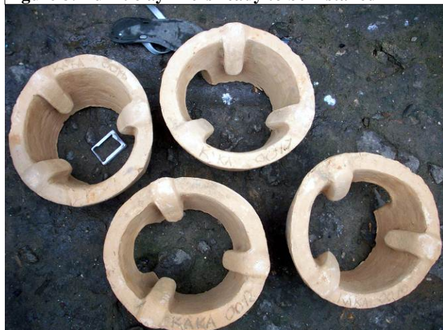
Figure 8: Burnt clay liners ready to be installed
