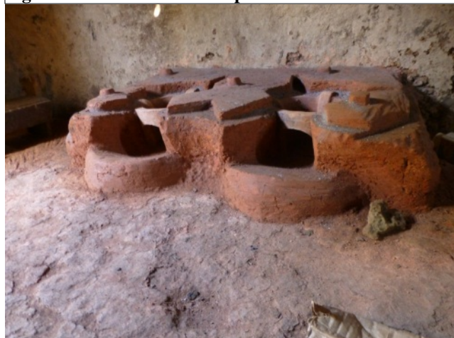
Figure 9: Finished Double Upesi-Stove
