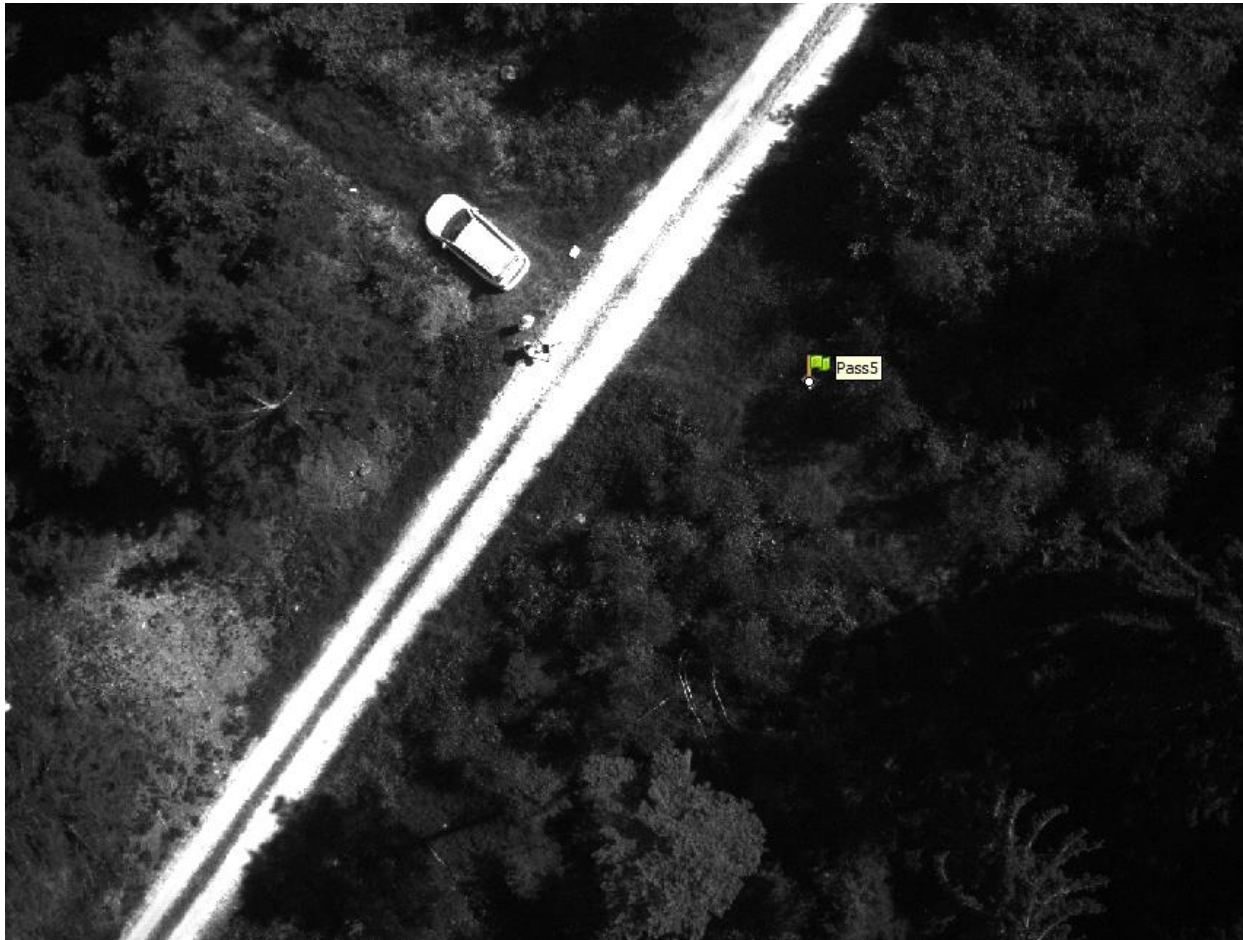
Fig. 9: Image from AIRPHEN 450nm band with a marked ground control point (GCP)
