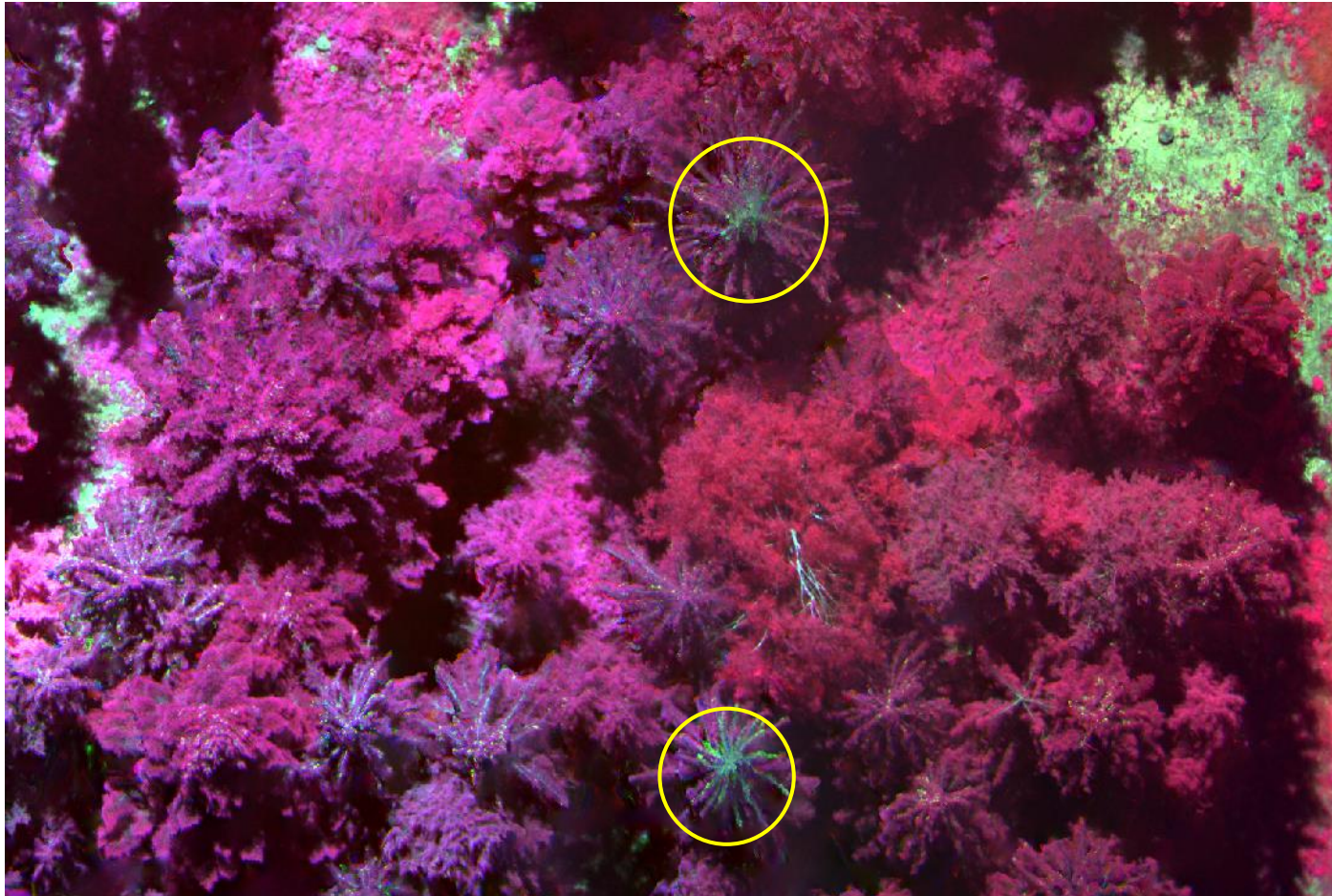
Fig. 19: Excerpt of Multilayer Stack with two stressed spruces (yellow marks)
